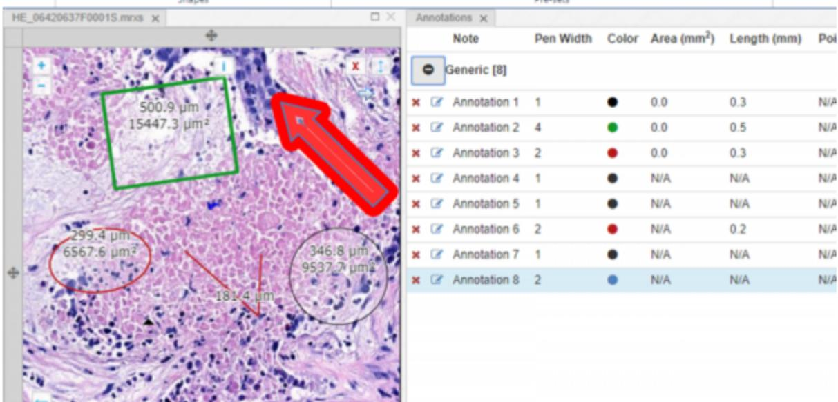
In the annotations panel, you see that area and length of annotation objects are calculated based on a dimensionality of the respective object. If you just draw a line, then the line by definition has no surface area. If you just put a landmark icon down, it has neither an area or a length.
